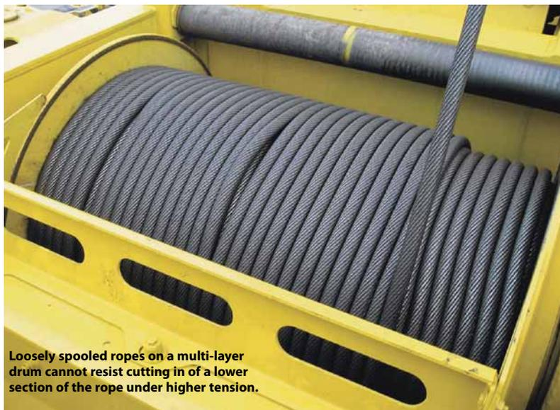
Loosely spooled ropes on a multi-layer drum cannot resist cutting in of a lower section of the rope under higher tension.
