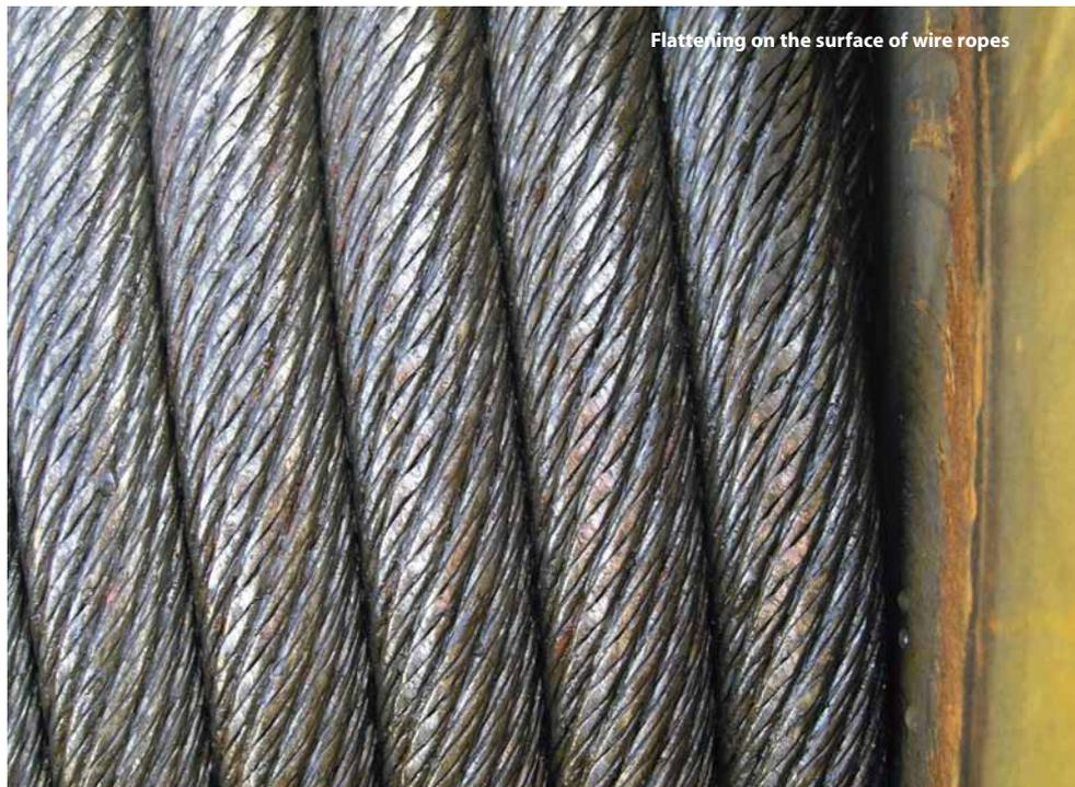
Flattening on the surface of wire ropes
